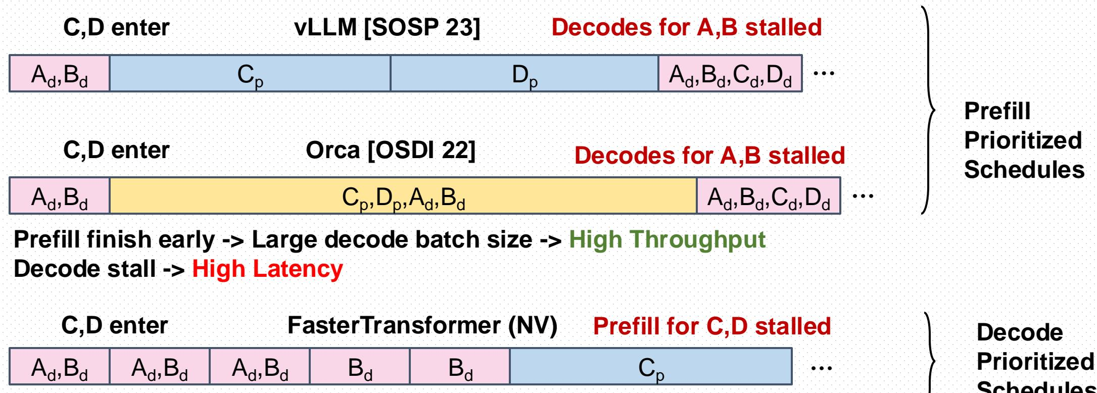
Decode without interference -> Low Latency
